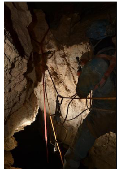
Figure 85: Tanguy Racine driving a spitz in the hard limestone wall - although lightweight, the complete handbolting kit comprises hammer, driver, spanner, spitz, hangers, cones and maillons - it's easy to forget one item!
