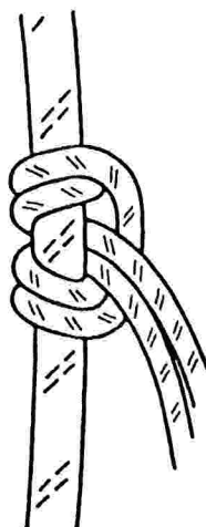
Prusik's Knot: 4 coils around the rope.
